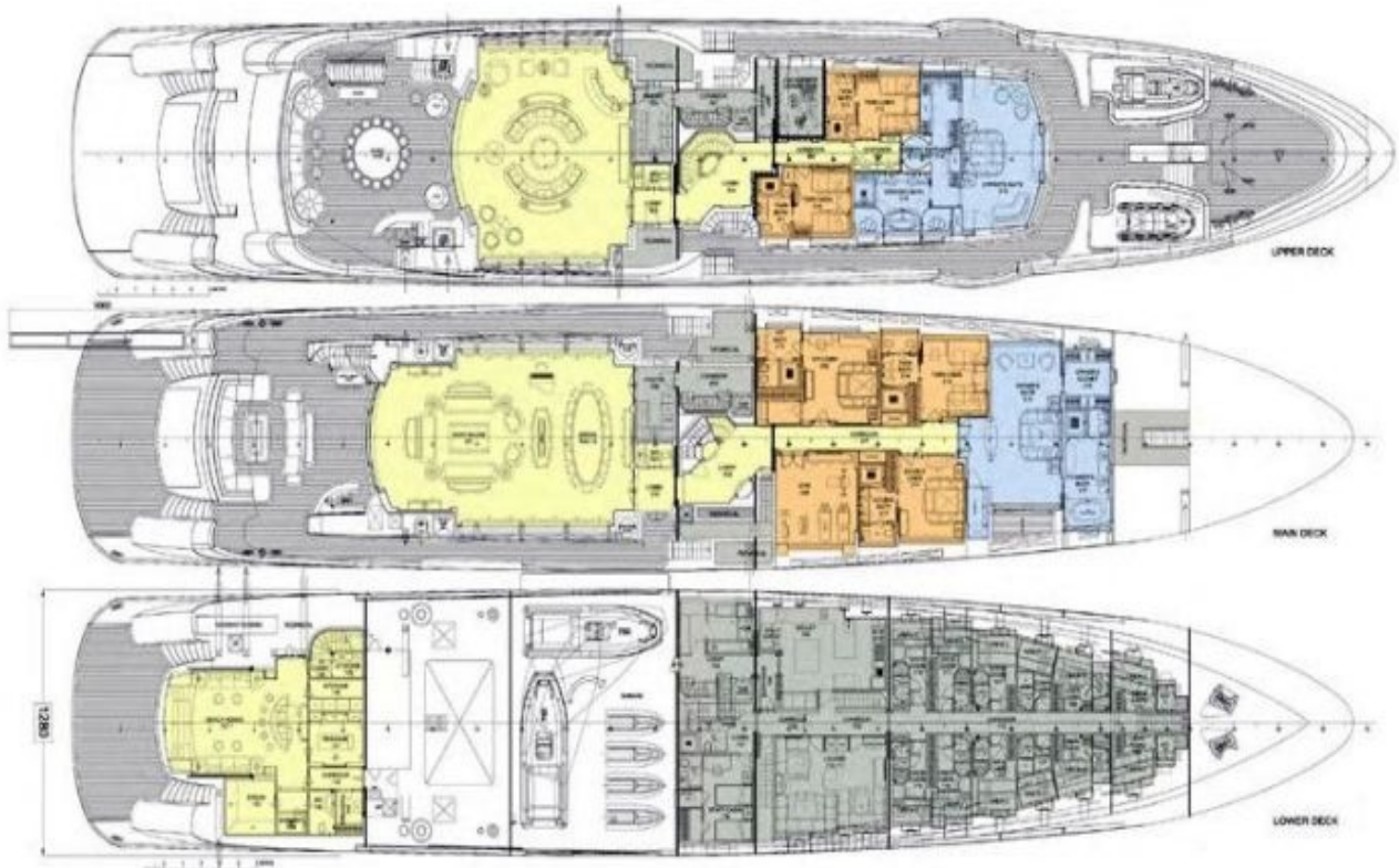
72 GOLD - LOWER MAIN UPPER DECK ACCOMODATION - SCALE 1:200
